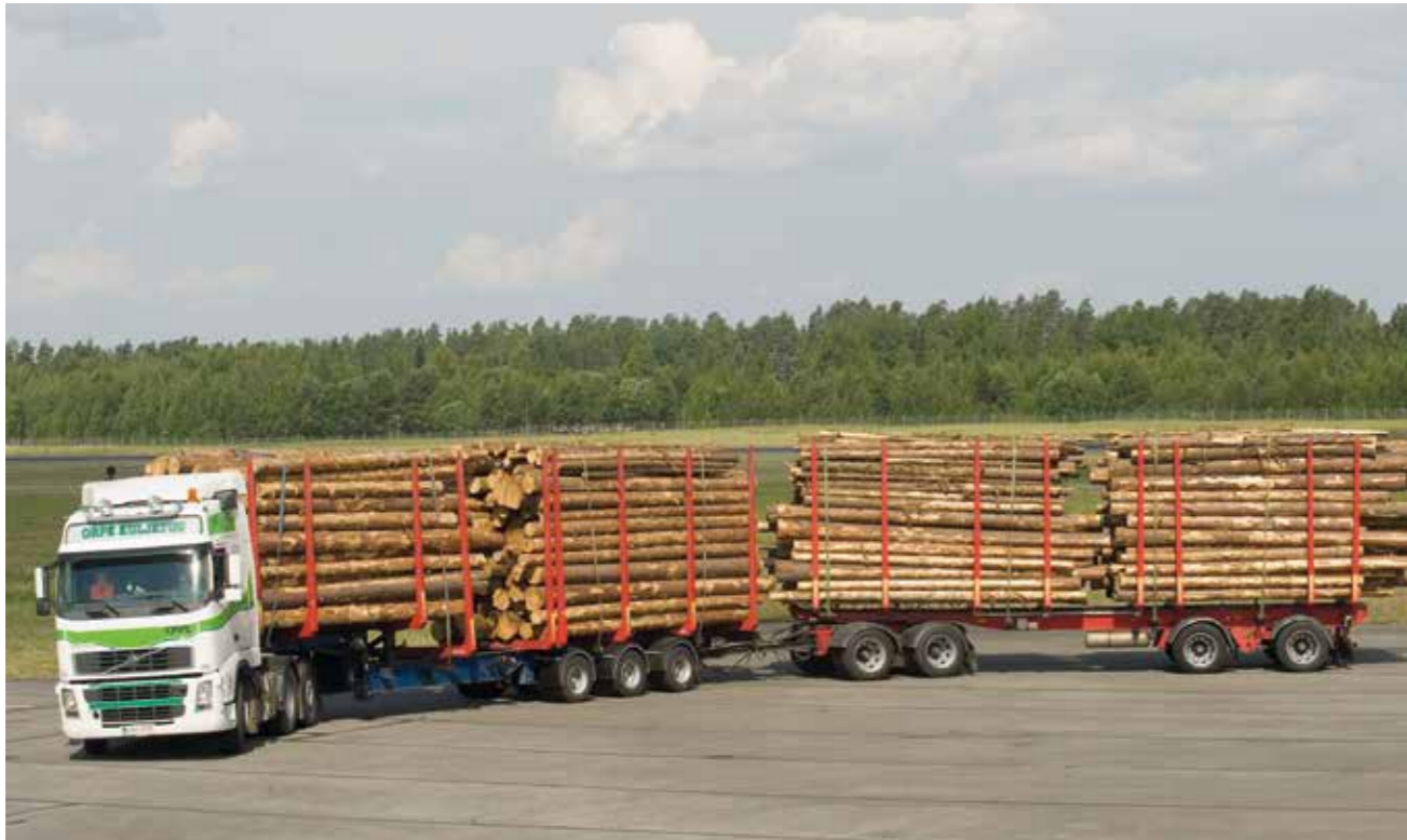
Photo 12. Pilot testing of a HCT vehicle at the Lappeenranta airport. (Photo: UPM)
