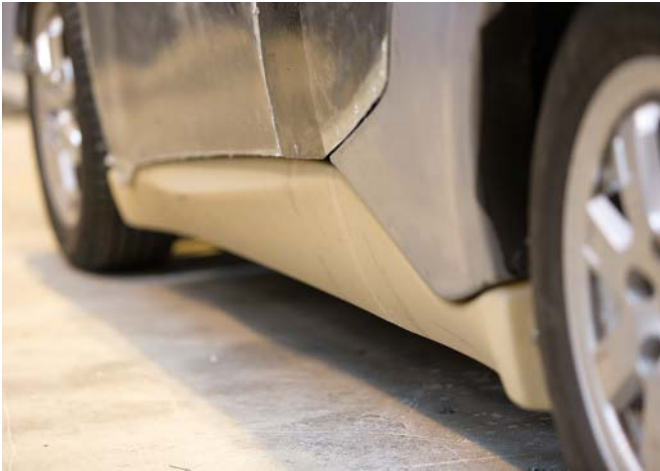
Ecological thermo-formable wood material replacing steel sheets in cars. (Photo: UPM Plc)
