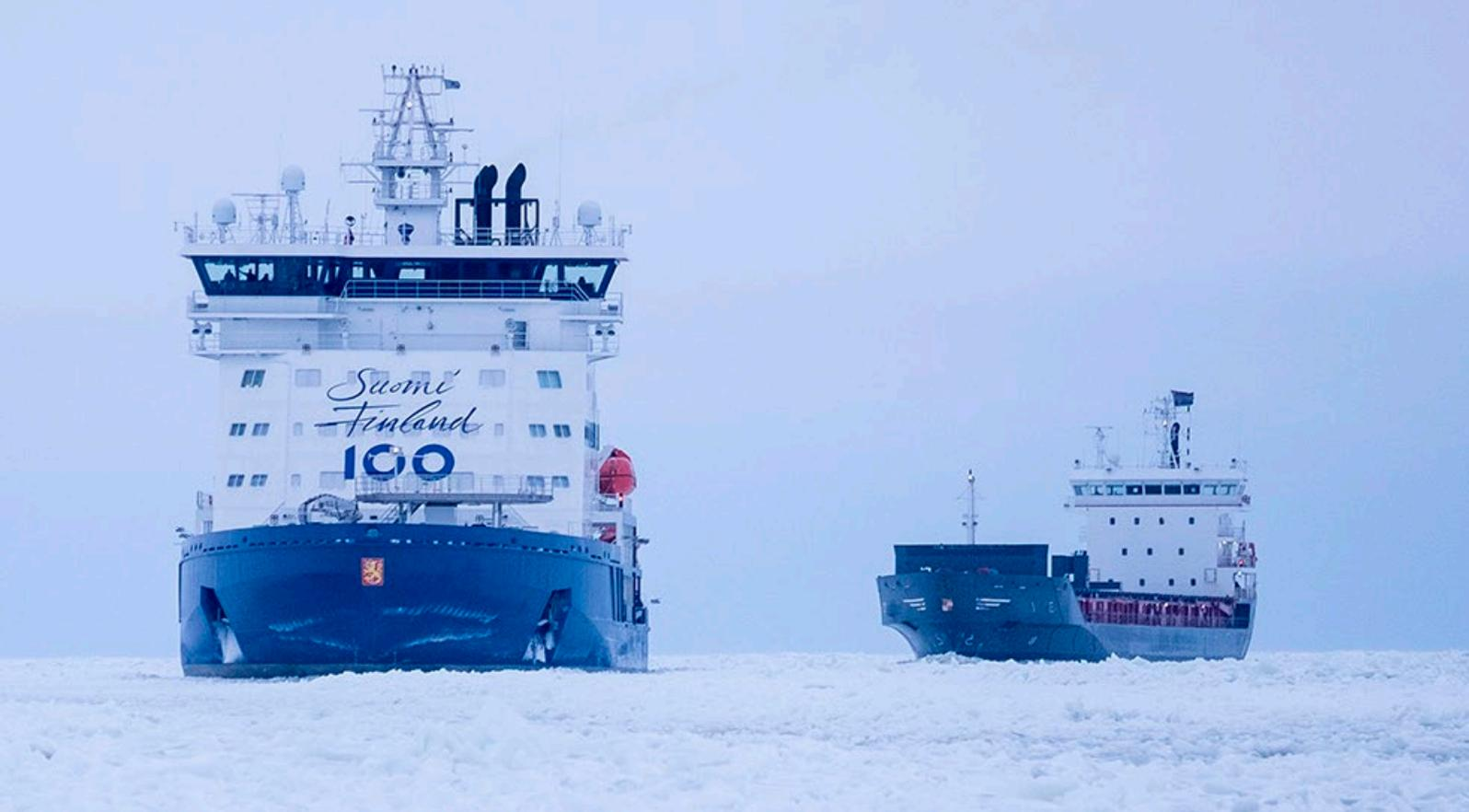
**Polaris, the first icebreaker in the world that can use liquid natural gas (LNG) as fuel as well as diesel. Photo: Timothy Bird**
