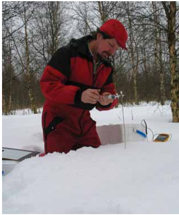
Taking a gas sample using the snow gradient method in a planted stand of birch trees on a former organic cropland (Photo: Jyrki Hytönen).
