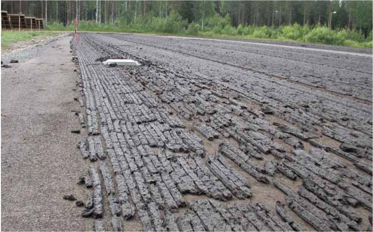
Peat harvested with a new peat production method on the peat drying field. Solar energy is utilized in the drying process (Photo: Sakari Sarkkola).
