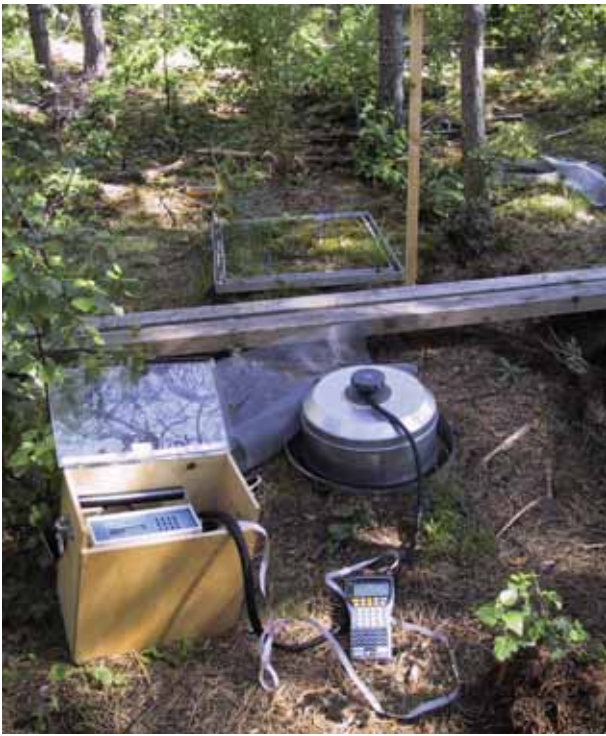
Soil respiration measuring equipment on an afforested organic cropland (Photo: Mikulas Cernota).
