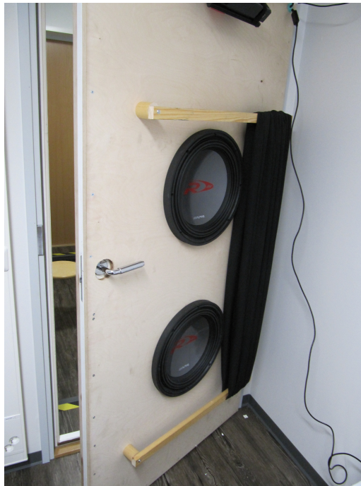
Figure 4.1: Loudspeaker drivers attached to the reinforced door of the measurement chamber were hidden behind a curtain during tests.
