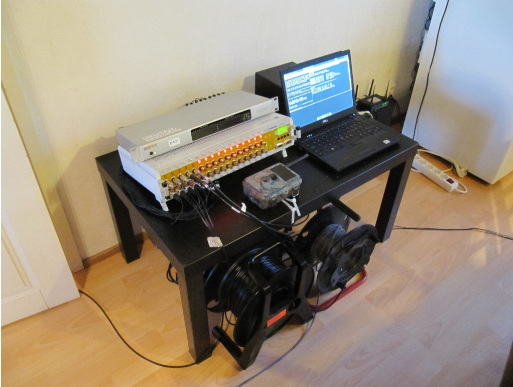
Figure 2.10: A five channel measurement setup streaming data from two microphones and a triaxial accelerometer to a cloud-based computational resource.
