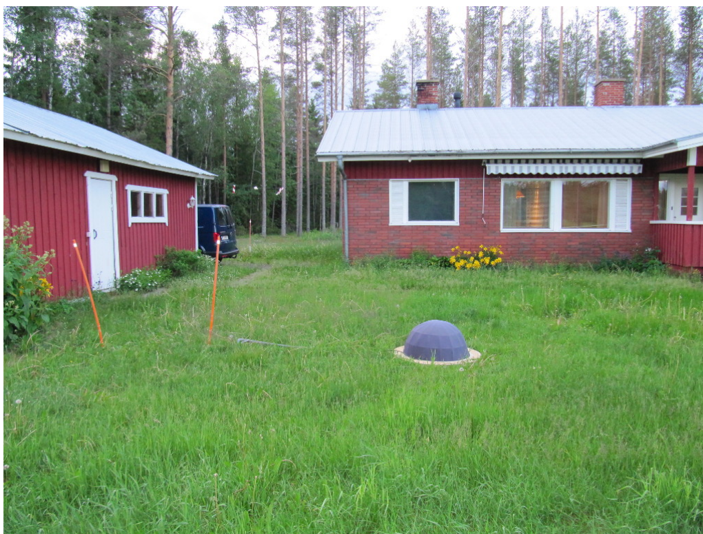
Figure 2.2: A view from the front yard of the house in Raahe. The outdoors infrasound microphone with a ground plate and a secondary hemispherical windshied of about one meter in diameter.
