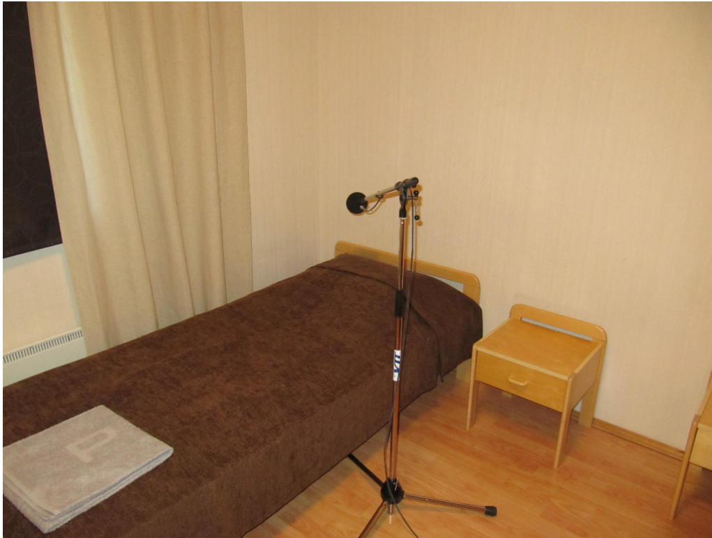
Figure 2.11: Indoors microphone positioned over a bed, a half metre above the head position.
