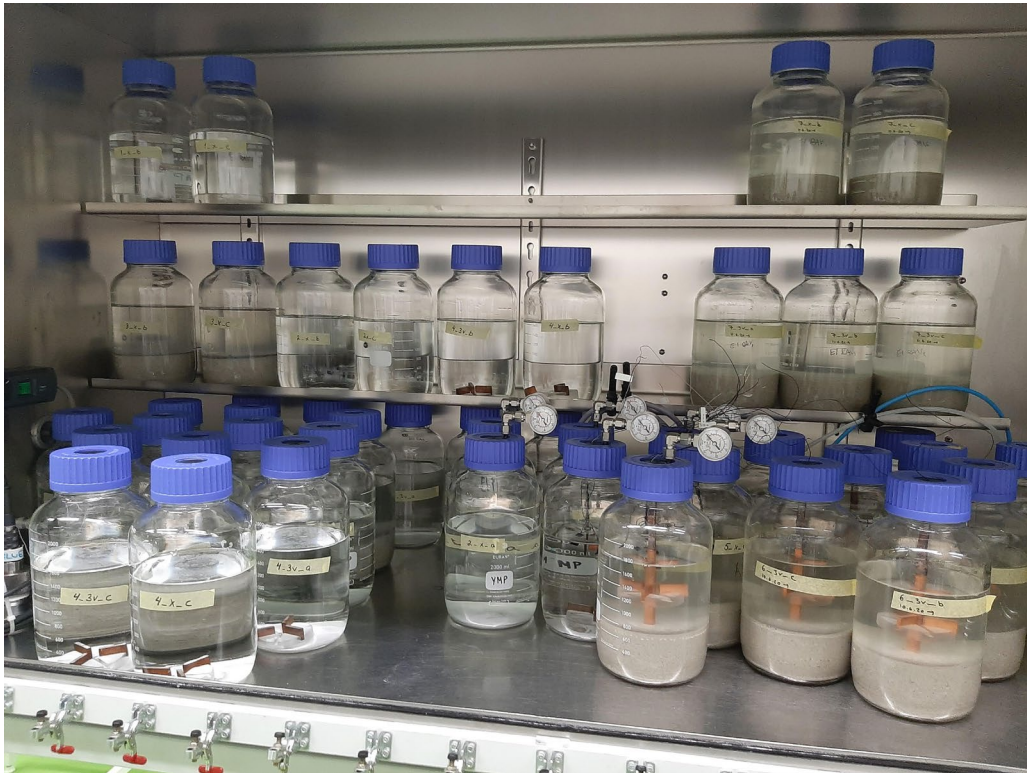
Figure 5.10. Multibarrier experiment simulating final repository conditions. On the left: Glass mesocosms with bentonite slurry, copper specimens and Olkiluoto groundwater. On the right: Reactors with compacted bentonite.
