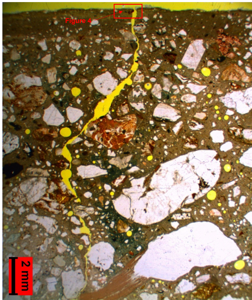
Figure 5.18. Petrographic thin-section analysis showing vertical crack extends through the sample depth, along the edge of the aggregates.
